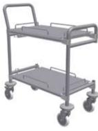
This cart is specially designed for transporting **particle sensing machines** around the cleanroom environment. Ergonomic design. Shock absorbing system in each wheel protects the valuable particle sensor from vibrations and shocks. Telescopic arm attached to cart allows sensor placement to a height of 3m. Jointed arms at the end of the telescopic arm enable positioning of sensor underneath hoods and in awkward places.
